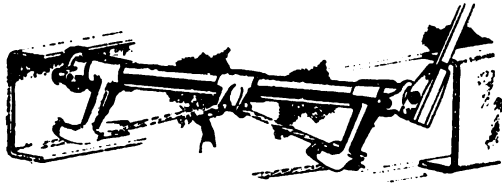
Side brake, shaft, and compensating device on Lanchester cars.
